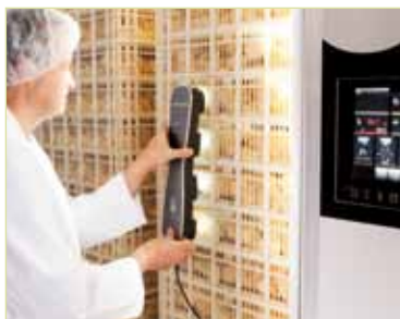
< Operator attaching a Synchro-Hatch™ embryo-response sensor
