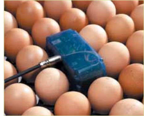
▲ OvoScan™ sensor positioned in egg tray
