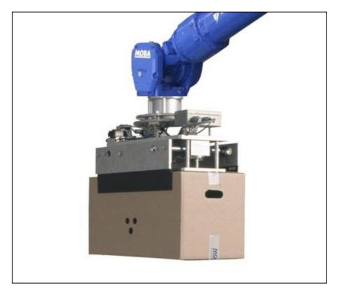
The multifunctional pickup head is able to handle empty pallets, layer pads and of course cases and crates.
